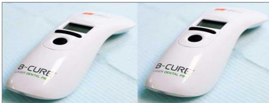
Fig. 1. B-Cure Laser Dental Pro portable dental laser therapeutic apparatuses: «active» - generating laser radiation, and placebo apparatus simulating laser beam generation.
